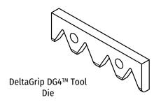
ASC Steel Deck's DeltaGrip® DG4™ Tool features a new four-tooth punch and a strengthened design, increasing deck connection strength and improving system durability. The improved connection performance make it a clear choice over traditional top seam welds and screwed sidelaps.
